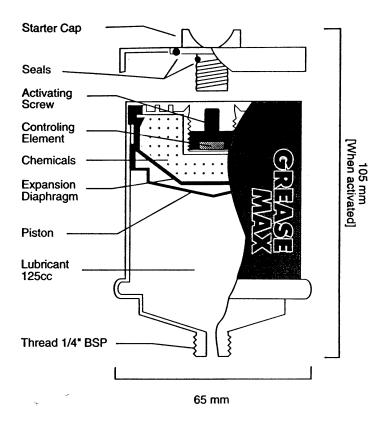
**GREASE MAX** <sup>®</sup> requires a minimum of approximately 8 hours for a type 1 unit to approximately 40 hours for a type 12 unit to develop sufficient internal pressure to commence discharging lubricant. This period is normally not a problem for well maintained bearings however if lubrication is required in less than the start up period then activate **GREASE MAX** <sup>®</sup> in advance.
